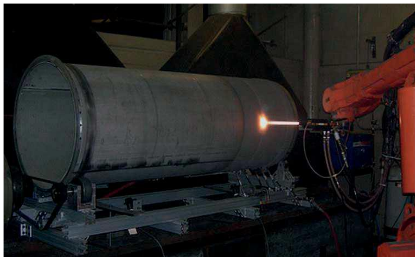
Fig. 8 High Velocity Oxy-Fuel (HVOF) process is used to coat a container with SAM1651 amorphous metal with quality assurance monitoring the thickness and roughness of BMG coating. [23]
